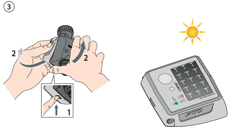
The timer can be disconnected from the control unit and just the timer can be positioned in direct sunlight.
