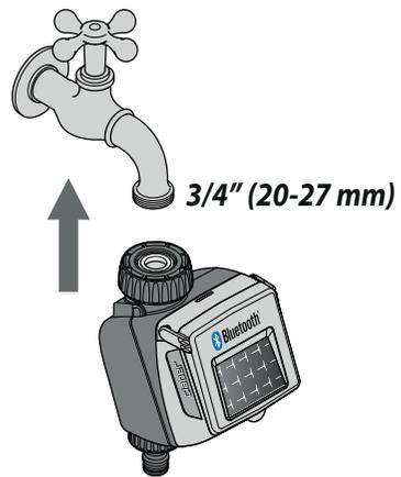
Fit the timer to a cold water tap. The spout of the tap should have a 3/4" male thread (if not, use an adaptor).
