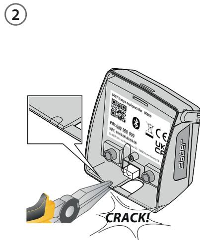
With the help of small pliers, break the plastic plug for preparing the slot of the Rain Sensor cable.
