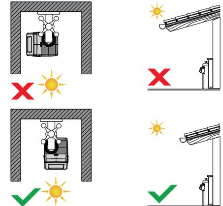
Once the timer is installed, make sure that the photovoltaic panel is pointed in the direction of the open area from which most light comes during the day. This is to ensure it charges correctly.
