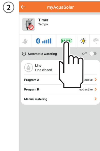
The energy level is also shown on the top toolbar after the timer profile has been opened. Selecting the energy level icon gives access to further information.
