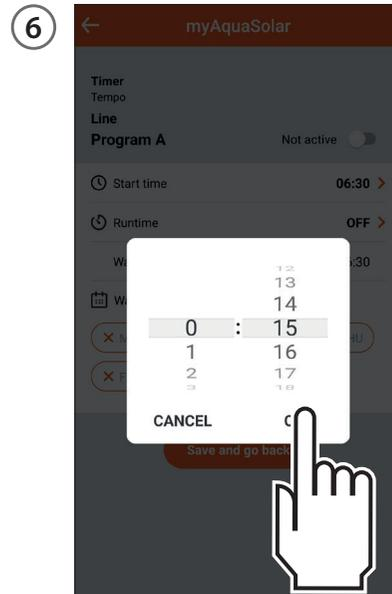
Scroll through the hours and minutes until you reach the run time you want and confirm. Watering can be set from 1 minute to 3 hours and 59 minutes.
