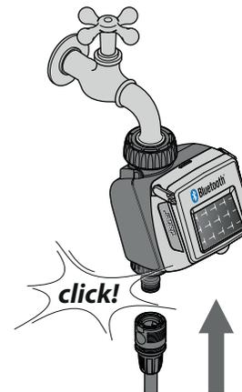
Connect the irrigation line to the timer connector using a Quick-Click System fitting or a 3/4" threaded fitting.
