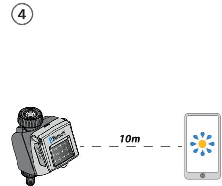
If the timer should run out of charge completely and turn itself off, it might start itself up again after normal exposure to the sun. If it goes off, the timer will lose the date and time setting: watering cycles might then start up in an abnormal fashion. If there is any suspicion that the timer might have been off, bring your smartphone to within 10 m of it to automatically update the date and time and, after checking that the Bluetooth® icon is blue, press the product profile in the app.
