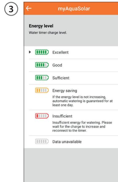
If the energy level icon is grey, wait for charging to be completed (FIRST OR NEW START-UP). There are 5 energy levels. If the energy level goes into **energy saving** (yellow icon), the timer will still guarantee automatic watering cycles for at least 1 day. When the energy level is **insufficient** (red icon), all the functions will be disabled. The date and time are saved in the memory for approximately 16 hours before the timer turns off.
