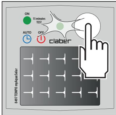
To activate manual watering from the timer, repeatedly press the Tempo myAquaSolar button until the LED flashes green. In this case, manual irrigation will run for 15 minutes.
