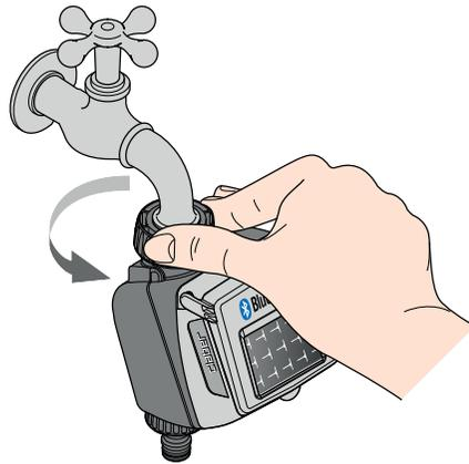
Screw the clamp collar of the 3/4" female fitting onto the tap. **Caution: tighten the collar using hand pressure only. Do not use wrenches or other tools**
