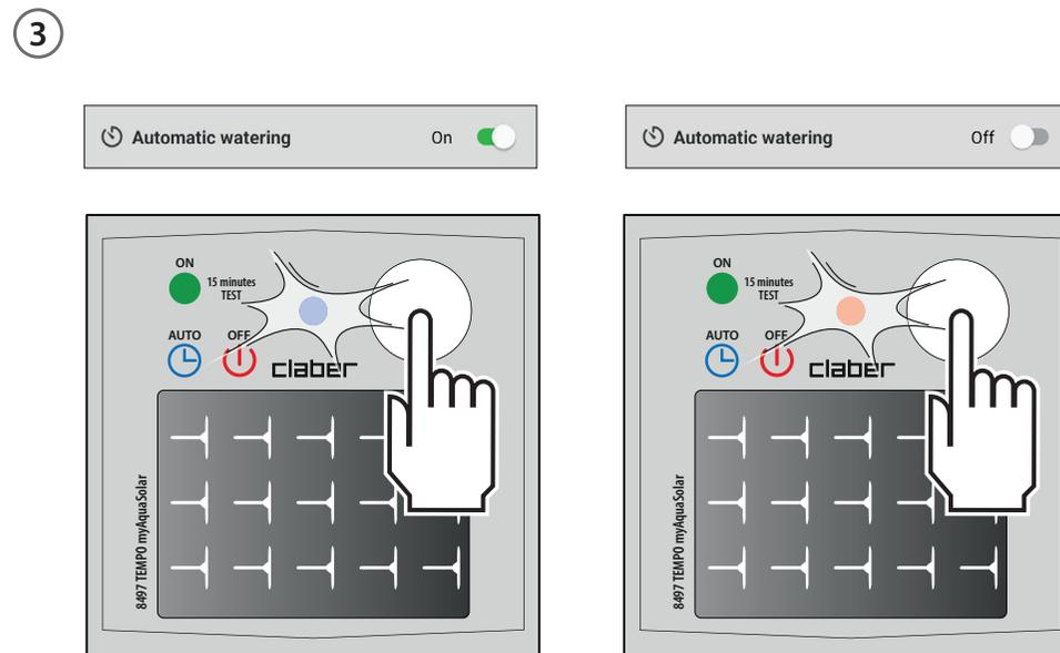
Press the timer key once to display the status. The automatic watering on status can be identified on the timer through the flashing blue LED; the automatic watering off status through the flashing red LED.
