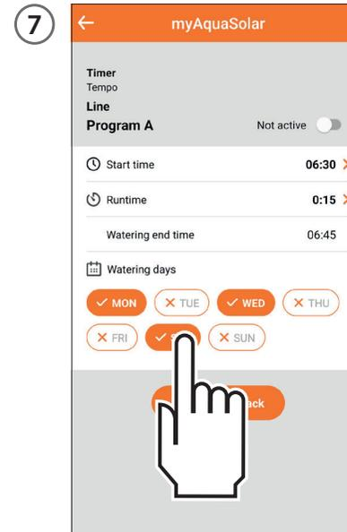
Then select the days of the week on which you want the irrigation cycle to run. Watering will take place on the days shown in orange.
