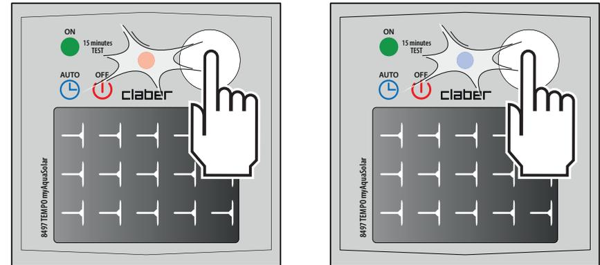
To pause it before it is finished, repeatedly press the timer key to set the desired status: automatic watering on (blue LED flashes) or no automatic watering (red LED flashes).
