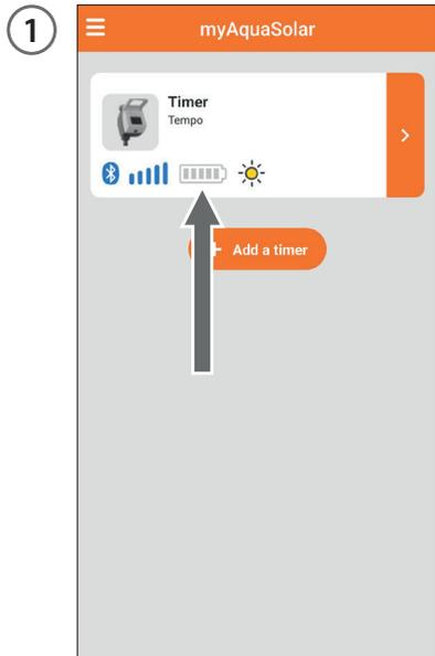
The timer will only be able to water if it has enough charge. To make sure it has the right charge before using it, check the energy level icon.
