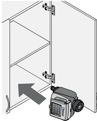
Store the timer in a sheltered place, away from damp, where the temperature does not fall below 3°C.
