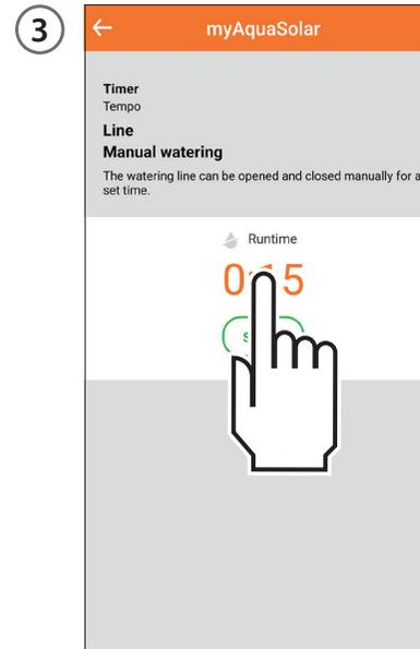
Press on the information about the watering run time to set the watering run time.
