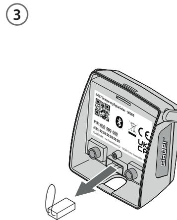
Remove the bridge connector on the timer.
