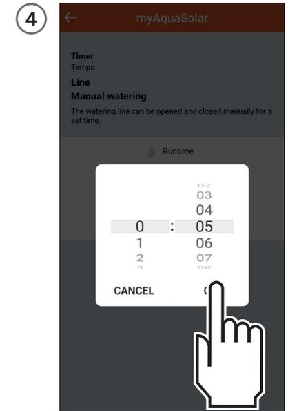
Scroll through the hours and minutes until you reach the run time you want and confirm. Watering can be set from 1 minute to 3 hours and 59 minutes.
