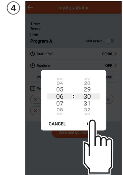
Scroll through the hours and minutes until you reach the time you want to start the irrigation cycle at and confirm.
