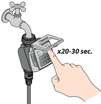
If the timer behaves anomalously, it can be reset. The reset will NOT cancel the programmes set, nor the date and time, but will only restart the circuit board.
