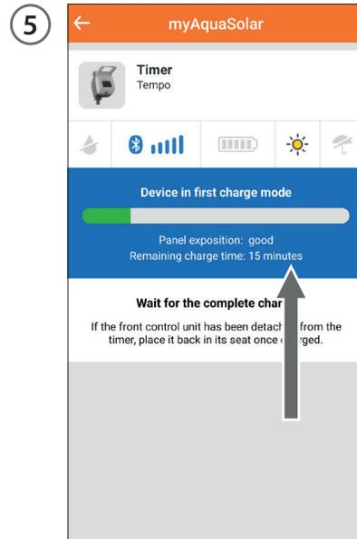
It will provide information about the charge status and the time remaining until charging is completed (from 30 to 90 minutes depending on how strong the light is).
