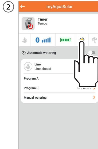
In order, the icons represent: watering in progress, Bluetooth® signal, energy level, solar radiation and Rain Sensor. Select an icon to find out what it means.
