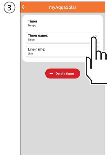
3 To give a name to the timer or the irrigation line, press the modification icon for the desired section. Enter the text and confirm.
